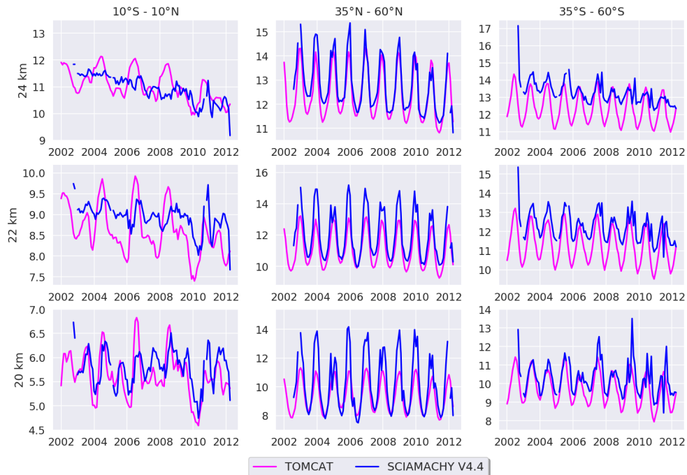
Figure 4: BrO volume mixing ratio (pptV) at different altitudes and latitudes from SCIAMACHY limb observations and TOMCAT model simulations.
